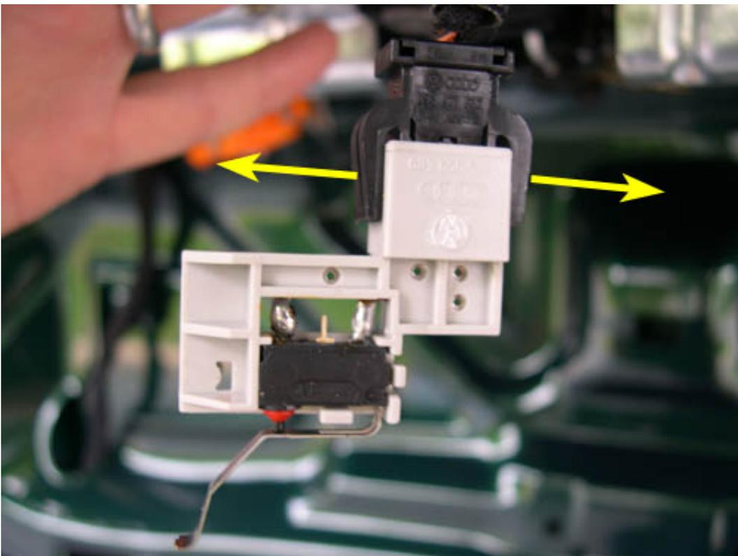
7. You can test to see if the microswitch is bad and causing the trunk light/dash indicator not to work by jumping the two terminals in the harness connector with a small wire. If the trunk light comes on, then the microswitch is bad and needs to be replaced. If the light doesn't come on, then the problem may also be somewhere else (but may be the microswitch as well). Check the bulb (you should really do this first) and the wiring between the harness connector and the light.
