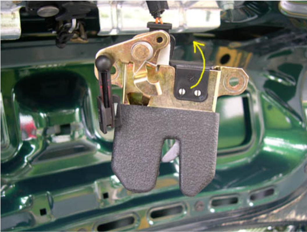
6. After doing so the microswitch should slide right out of the latch assembly, as seen in the picture below. Disconnect the microswitch from its harness connector by pulling the two side tabs outward (yellow arrows) at the same time.
