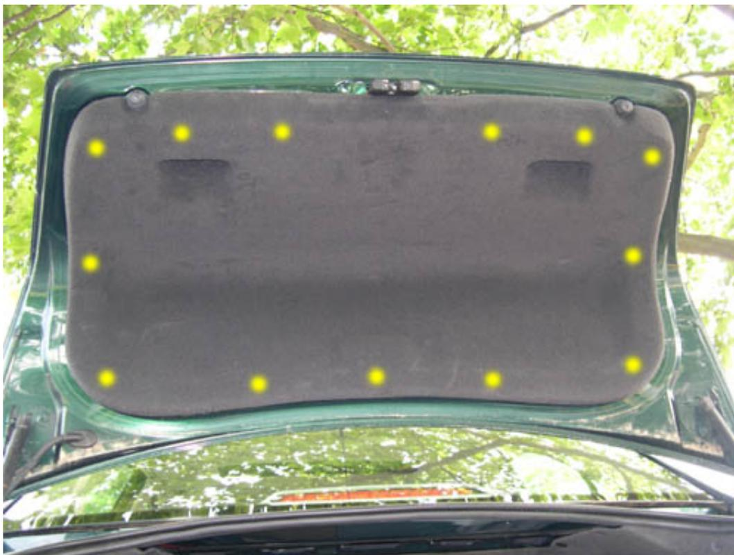
2. The screws in the above picture are coated with carpet fibers, so using a bare screwdriver may scratch the coating off. I used a ZipLoc Freezer bag folded in half to prevent this from happening, as shown below. It did a pretty good job of keeping the screw coating intact.
