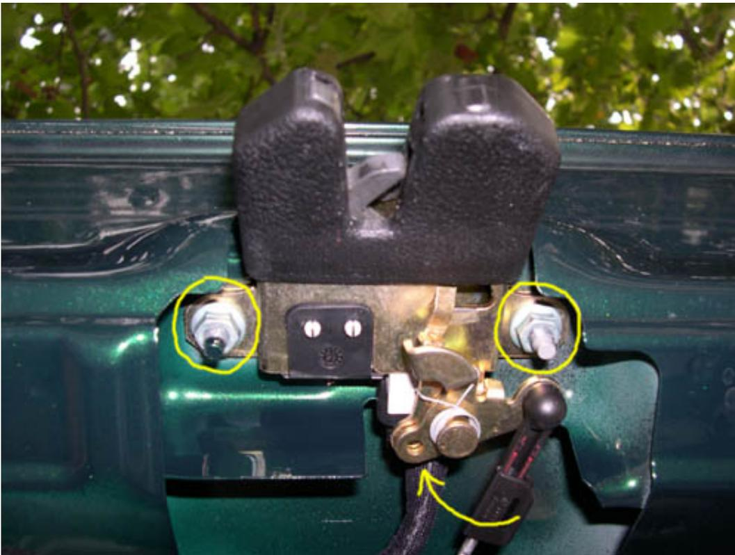
4. Remove (2) 10mm nuts (inside yellow circles in above picture) to disconnect the latch assembly from the trunk lid.
