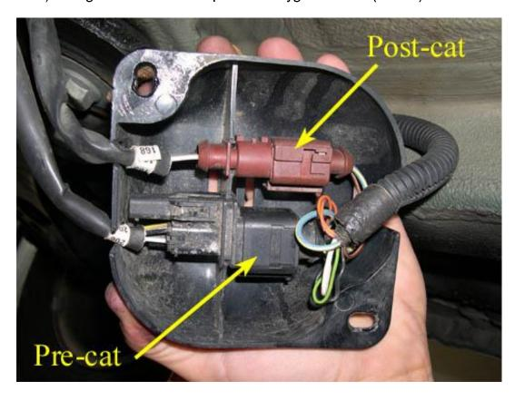
9. Separate the appropriate harness connector(s) by pulling up slightly on the retaining tab (indicated by the yellow arrow in picture below) with a screwdriver or other small, thin tool and sliding the two halves apart.
