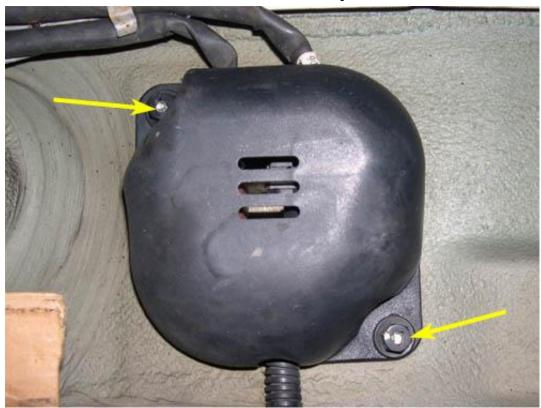
8. The picture below shows the sensor lead harness connectors inside the black plastic box. The harness connectors are attached to the box by tabs on either side of each harness connector. Slide the appropriate harness connector(s) off of the tabs to disconnect it from the box (this can be difficult to do - the fit is very tight). Note that the harness connector for the pre-cat oxygen sensor (6-wire) is larger than that of the post-cat oxygen sensor (4-wire).
