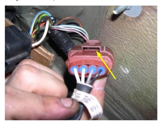
10. Remove the protective heat shield from around the sensor leads by unsnapping the snaps indicated by the yellow arrows in the picture below (there are approximately 4-5 snaps).
