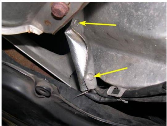
11. Remove the appropriate sensor lead(s) from the retaining clips on the underside of the car. One of the clips is indicated by the red arrow in the picture below.
