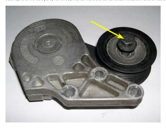
8. The picture below shows the pulley removed from the tensioner unit. Note that there is a pulley guard (top center of picture) that is used between the bolt and pulley.
