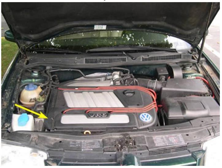
2. Remove the long cover piece on the passenger's side of the engine to reveal the tensioner. To do this, remove the two (2) T30 Torx screws (indicated by the yellow arrows in the picture below) and carefully pull upward on the cover piece.
