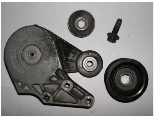
9. Use a small screwdriver to remove the seals from each side of the pulley bearing, as shown in the picture below. To do this, insert the screwdriver between the seal and inner race and VERY CAREFULLY pry the seal upward. Make sure you do not damage the rubber coating on the seal or it may not stay in place when reinstalled.
