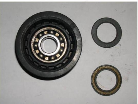
11. Pack each side of the bearing with some high temp. wheel bearing grease or another suitable lubricant, as shown in the picture below. You can also add a drop or two of oil to thin out the grease if it's very thick.
