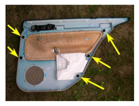
9. Starting with the top, rear corner, pull the door panel up and out of the window seal, as shown below.
