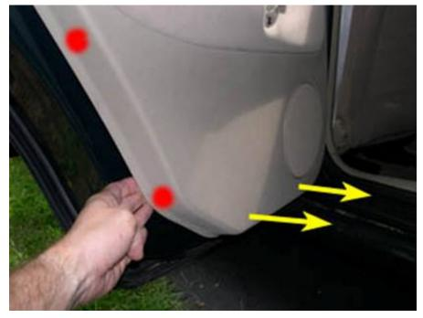
8. The picture below of the inside of the door panel shows the location of the five snaps. (This picture is for reference only and was taken later in the DIY. The door panel should not be off yet).
