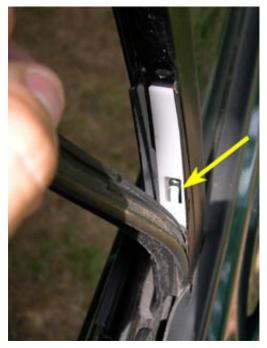
21. Using a screwdriver, pull the tab outward and simultaneously slide the insert up and out of the door, as shown below.
