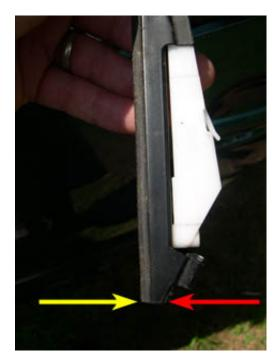
24. Installation of the new insert is the reverse of the above. The tab on the new insert should click into place if installed into the door correctly.
