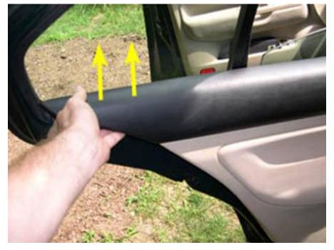
10. Do the same with the top, front corner of the door panel, as shown below. The door panel should now be disconnected from the door except for the electrical and door lock cable connections in between the panel and the door. You can rest the door panel back into the window seal if you want to take a break or reach for a tool.
