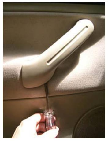
3. Once one end of the outer handle piece is pried off slightly, move to the other end and pry that out slightly, as shown below. Go back and forth between ends until the handle has been pried out approx. 1/8". Once it is this far out, you should be able to pull it off the rest of the way with your hands.
