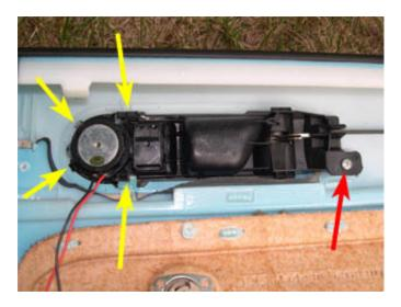
16. Once the front edge of the handle assembly is pushed out (1), slide the assembly toward the front of the car to remove (2).
