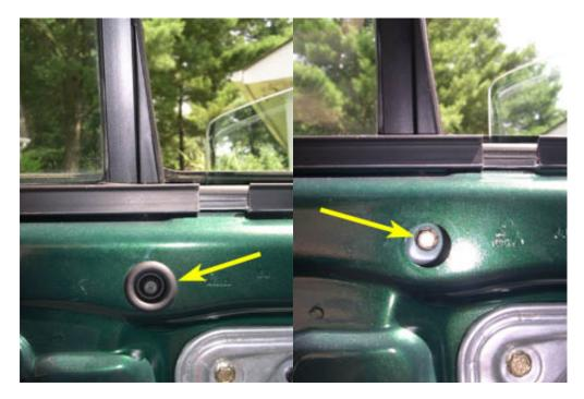
19. Pull the rubber window seal away from the insert, as shown below.
