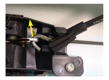
13. The picture below is a side view of the cable retaining clip to help illustrate how to detach it. You need to pull outwards on the front of the clip (1) to clear the tabs and then slide it to the rear (2).
