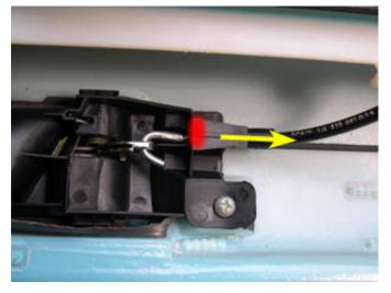
12. Once the clip is unhooked, remove the cable from the groove in the unlock handle assembly and then detach the hook from the unlock handle, as shown below.
