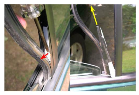
22. The picture below shows the entire insert still attached to the rubber window seal.
