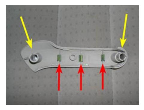
5. The picture below shows the inner handle piece still attached to the door panel. The handle piece is attached to the door panel with three medium Phillips screws (red arrows) and the door panel is secured to the door with 2 large Phillips screws (yellow arrows). If you want to remove the inner handle piece from the door panel, remove all five screws. If you are just taking the door panel off, only remove the two large screws indicated by the yellow arrows.
