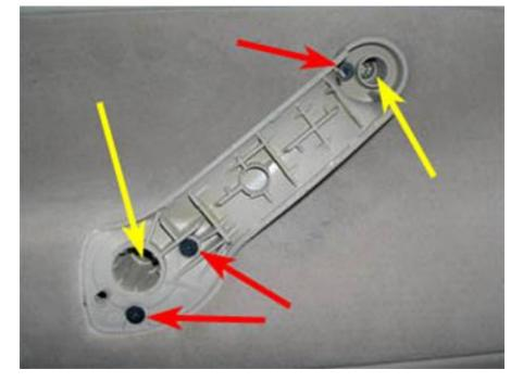
6. Remove the two T20 Torx screws at the bottom of the door.
