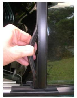
19. Pull out the seal from nearly top to bottom, as shown below, but don't remove the seal completely. Leave it attached at the top of the window and also to the bottom of the triangular insert. This will help insure that it goes back in correctly.
