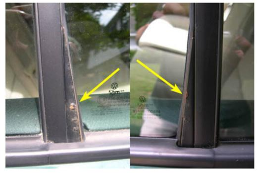
18. To remove the inserts, begin by removing the rubber grommet on the door just below the insert and then removing the 10mm bolt behind it, as indicated below.
