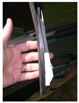
23. Take note of the position of the bottom of the rubber seal (yellow arrow) relative to that of the bottom of the insert (red arrow), as shown below. Make sure to attach the seal to the new insert in the same position so that the seal reinstalls into the quarter panel window divider correctly.
