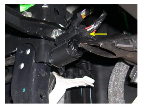
WARNING: If at any time during steps 5 and 6 the switch backs away from the bracket (even a little bit), DO NOT ATTEMPT TO ROTATE THE SWITCH INTO POSITION!!! It will
