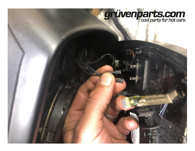
Now gently unclip the wiring associated with the mirror glass. There are usually 2 small black heater wires, then a wire plug. Unclip all and store the mirror glass in some bubble wrap.
