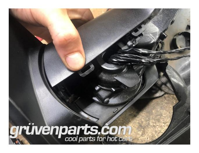
Step 5: Remove the metal drive arm by removing the 2 long torx screws that go thru the power fold drive unit. Wiggle the metal arm up and off of the power fold drive unit.
