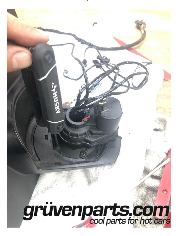
Step 7: Cut the plastic case just below the witness line where the upper and lower case halves were originally fused together. See Red Line in the picture below. You can use a small cutter such as a Dremel tool to do this. DO NOT Cut too deep. Work slow and cut just enough to separate the case halves. IF you cut too deep you will damage in the internal components. You can use a thin feel gauge to see if your cut has gone thru the case wall.
