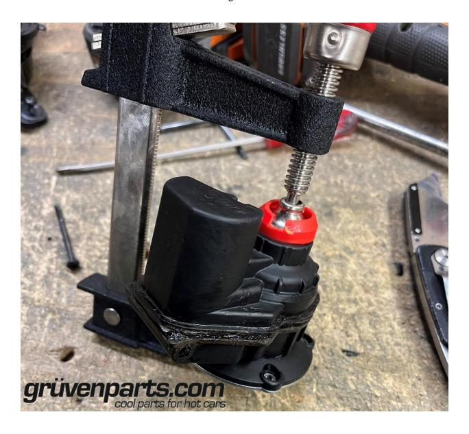
Step 11 – Reinstall drive unit into mirror assembly using the reverse procedure as disassembly
