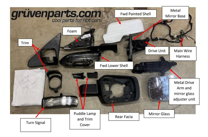
Please note that the mirror assembly doesn't need to be removed from the vehicle and no interior components need to be taken off. The entire job is handled on the outside of the vehicle. These pictures are taken in a shop with the unit off the vehicle but in the field the mirror will be serviced on the vehicle.
