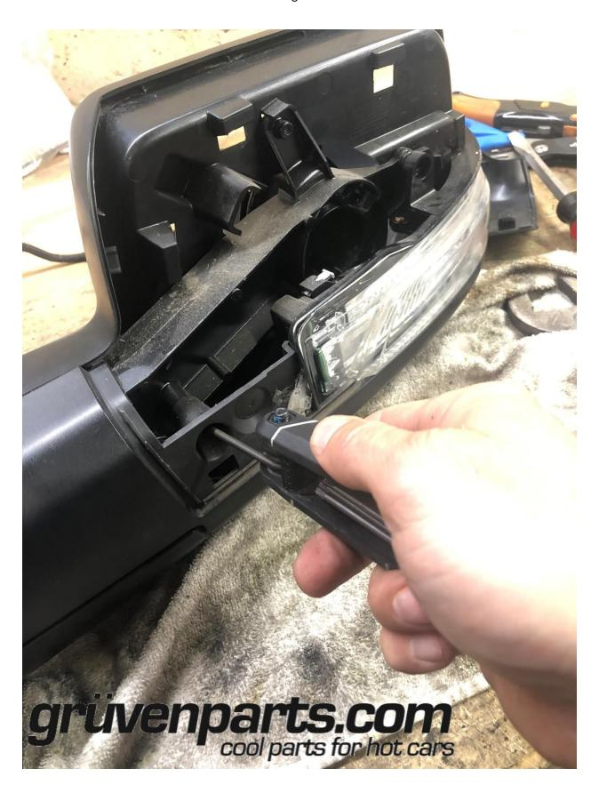
Step 4: Remove forward lower trim to expose the power fold drive unit. You can just unclip the tabs holding this in place carefully.
