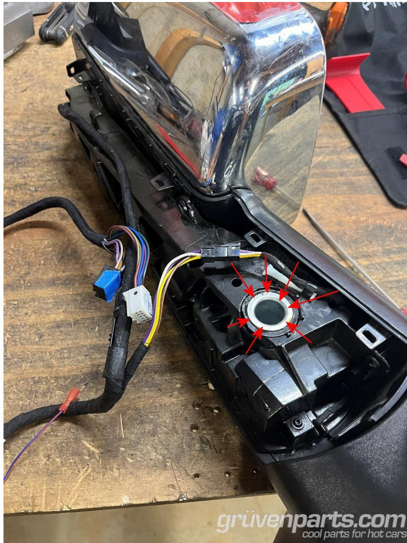
Figure 3 – Location of Small Cuts to the Return Flange on the Power Fold Pivot Tube
