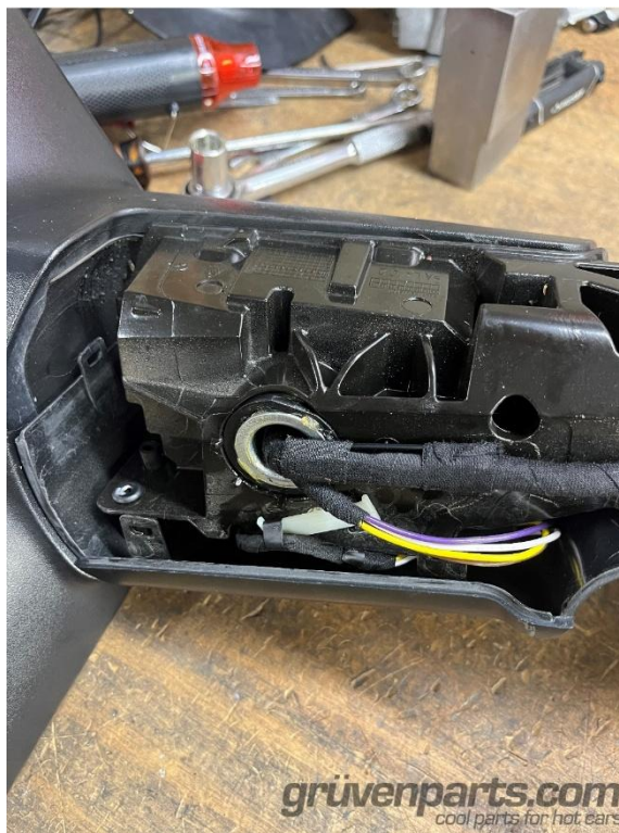
Figure 1 – Main Wiring Running Thru the Power Fold Pivot Tube
