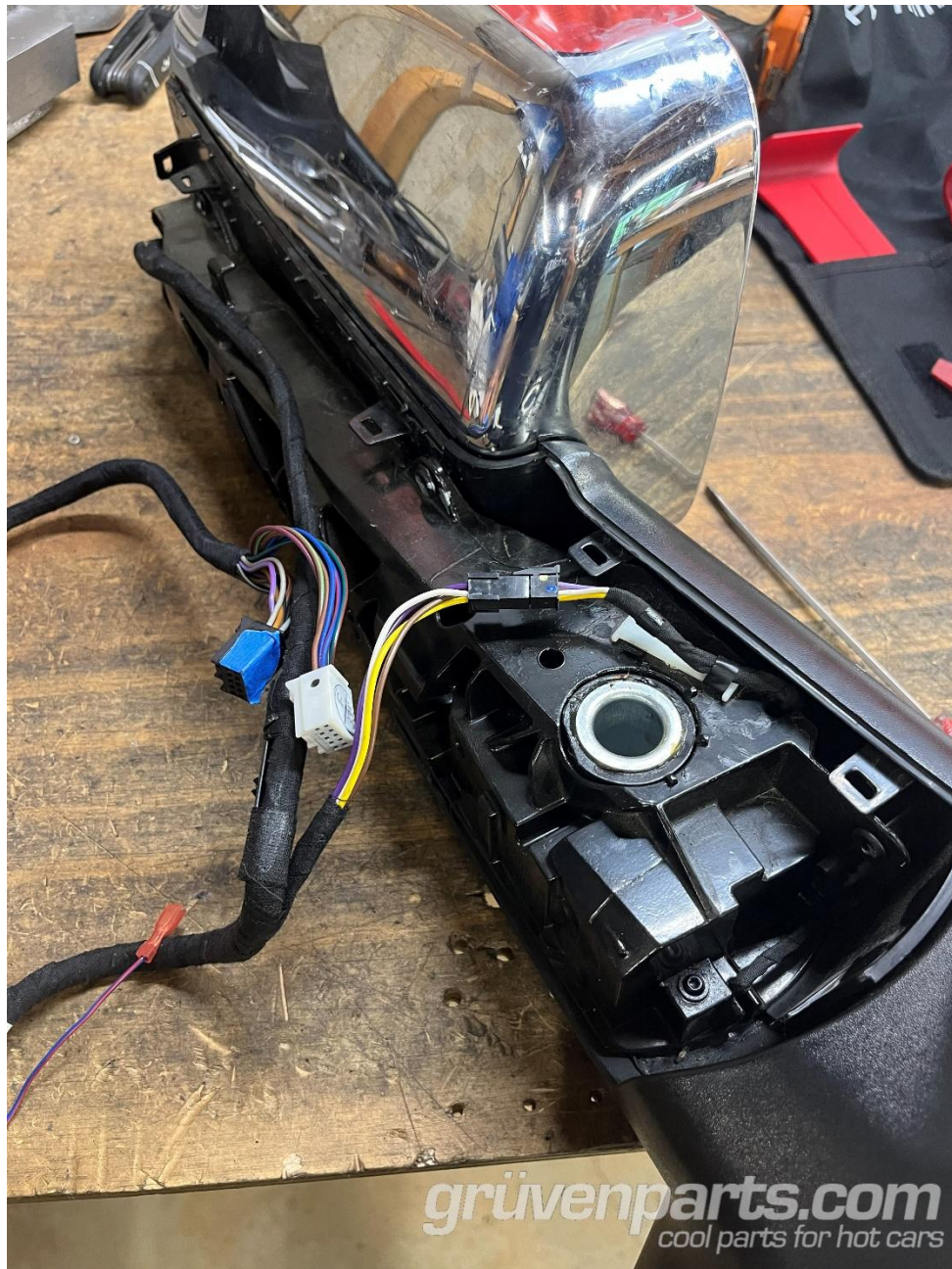
Figure 2 – Wiring Harness Pulled Back Thru Mirror Power Fold Pivot Tube
