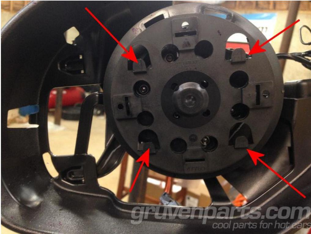
Mirror mounting base, mirror is removed in this picture. View looking aft. Arrows show the mating tabs which the mirror clips onto. When reinstalling mirror, align tabs and push mirror down onto tabs until a click is heard.
