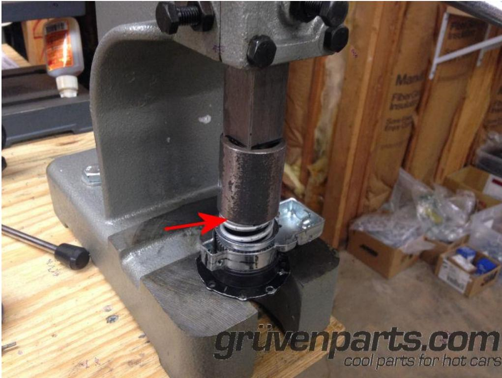
Arrow showing the retaining ring sitting just above the spring. You need to compress this and rotate the socket or collar about 1/6 turn either direction to disengage the retaining ring. Release compression slowly as the spring is heavy. You can also do this by hand with a deep well socket, by pressing down firmly on the spring then rotating. **Use eye protection and be careful, the spring is heavy.**
