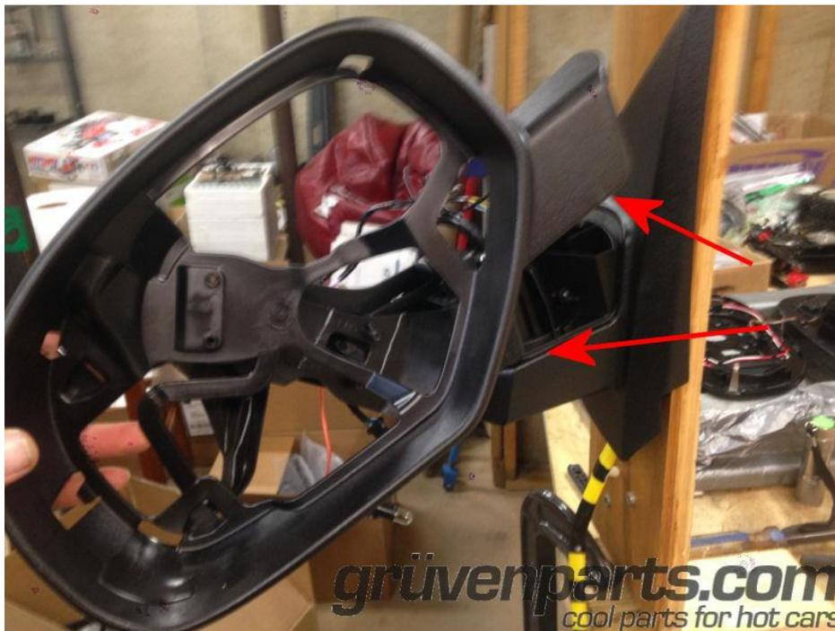
Mirror Frame unsnapped from mirror assembly. It can be set aside at this point.
