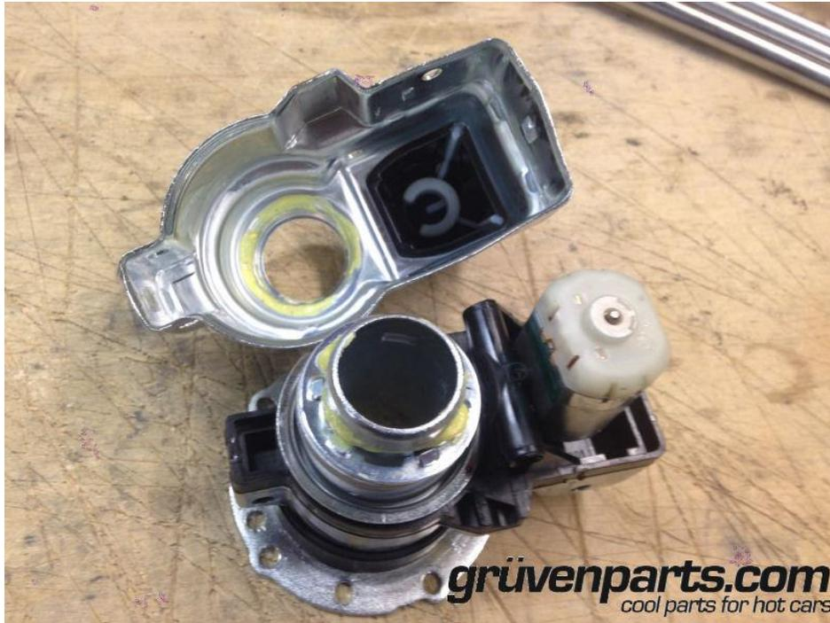
Case halves separated. Note motor on the right. Motor can be gently pulled straight up to disengage from the motor drive unit, or wait until main spring is removed and it will come up.
