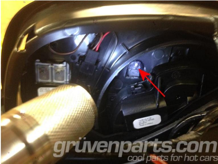
Arrow shows 1 of the mirror tabs, mirror installed looking at back side of mirror.
