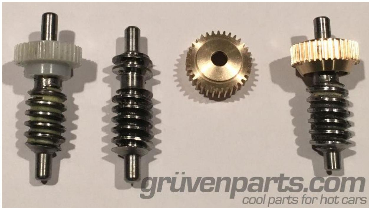
OEM main worm shaft with over-molded plastic spur gear show on the far left. OEM main worm shaft 2<sup>nd</sup> from left shown with plastic spur section removed. GruvenParts.com brass spur gear shown 2<sup>nd</sup> from right. GruvenParts brass spur gear shown installed via 24 hour JB Weld epoxy on far right.
