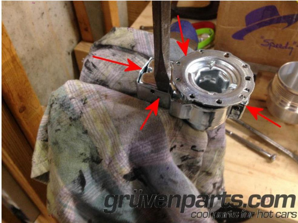
(4) Arrows show the locations of the snap fits. Flat head screw driver is inserted between the case halves, forcing outer half outward. Gently tap flat head screw driver downward to force case walls outward. Pry center portion upwards to separate.
