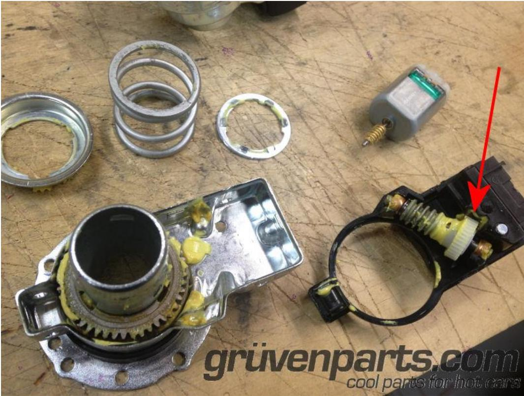
Discrepant gear shown. Note the plastic spur gear over-molded onto the metal worm gear. This is what has likely broken if you hear the motor whirring or if nothing happens when you hit the button. Most times the gear breaks apart and lodges into the unit, preventing anything from happening.
