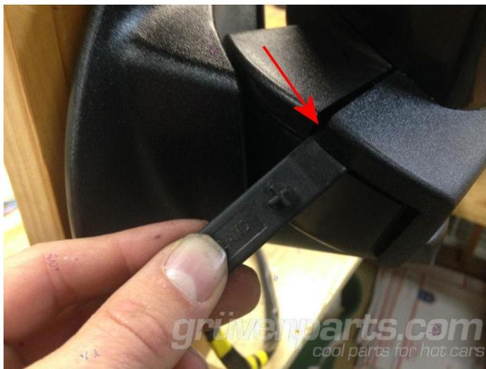
Slowly and gently work around the mirror shroud and remove both upper and lower plastic shrouds as 1 piece. You use hand force here, perhaps some gentle prying with the plastic lever.
