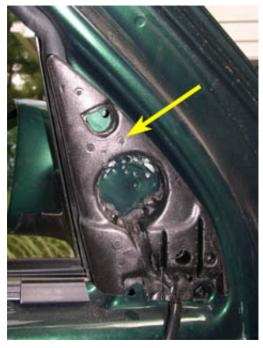
29. The sideview mirror assembly is attached to the door with a single T45 Torx screw (thanks bluetoyota for the size). Remove this screw and pull the mirror assembly off of the door - be careful not to harm the wires for the mirror glass heater element and the mirror motor.
