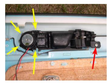
25. Once the front edge of the handle assembly is pushed out (1), slide the assembly toward the front of the car to remove (2).
