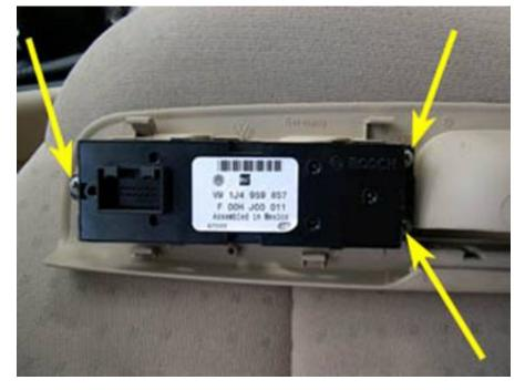
8. Remove the three large Phillips screws indicated by the yellow arrows in the photo below.
