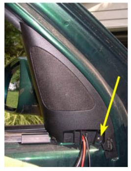
27. Pull the speaker grille off of the door. The inside of the grille is also attached to the door by three tabs which are indicated by the arrows in the picture below.
