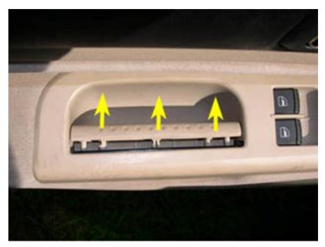
5. To take the main handle piece off of the driver's door panel, pull the rear of the handle upwards to unclip it, as shown below. Do the same at the front edge of the handle.
