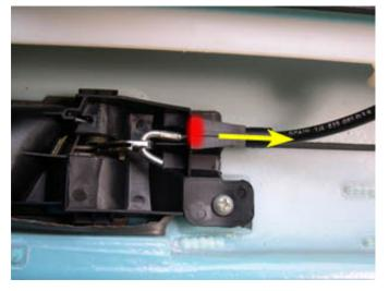
21. Once the clip is unhooked, remove the cable from the groove in the unlock handle assembly and then detach the hook from the unlock handle, as shown below.
