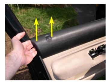
19. Do the same with the top, front corner of the door panel, as shown below. The door panel should now be disconnected from the door except for the electrical and door lock cable connections in between the panel and the door. You can rest the door panel back into the window seal if you want to take a break or reach for a tool.
