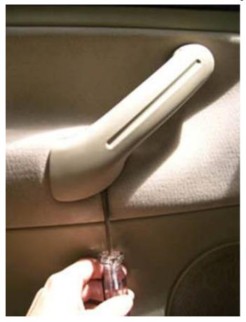
11. Once one end of the outer handle piece is pried out slightly, move to the other end and pry that out slightly, as shown below. Go back and forth between ends until the handle has been pried out approx. 1/8". Once it is this far out, you should be able to pull it off the rest of the way with your hands.
