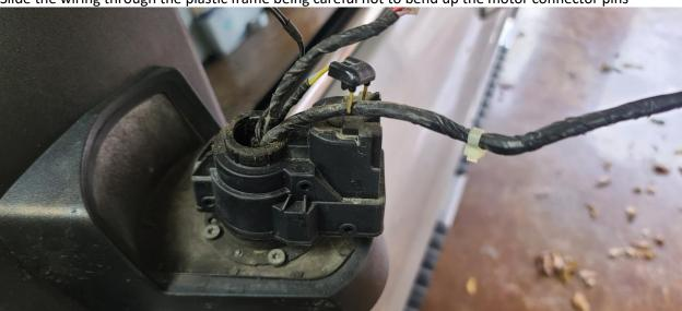
Note the location of the square in the lower motor housing in relation to the motor position and mirror mount
