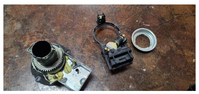
Carefully remove OEM circuit board/motor and install the new GruvenParts motor into OEM circuit board.
