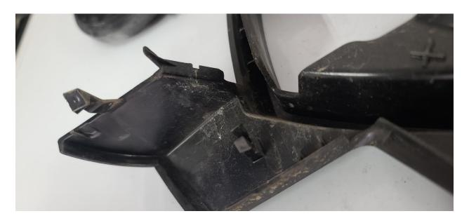
Unlatch the mirror puddle light and remove the connections
