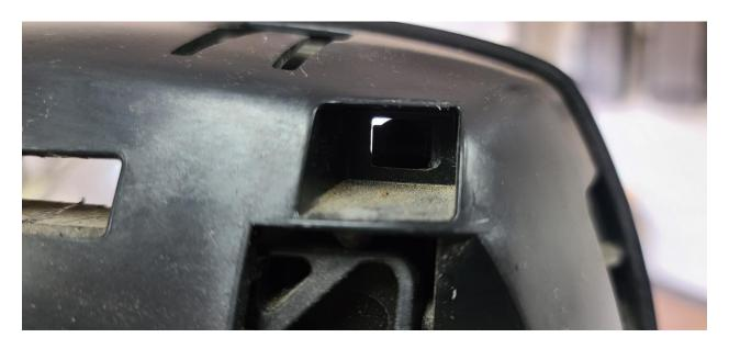
The 3 latches closest to the motor disconnect pretty easily with a trim tool and some wiggling
