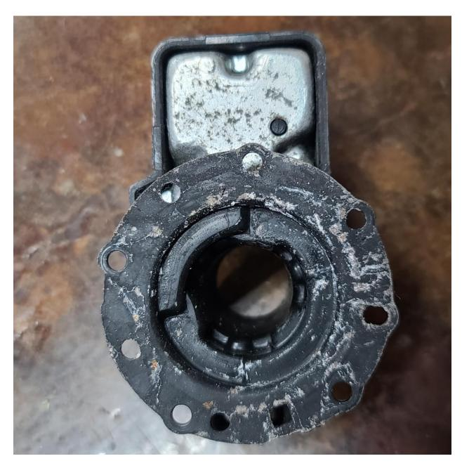
The motor cover is plastic and held on by 4 latches. I find it easier to clamp the lower motor mount in the vice and use small screw drivers to gently lift the latches while pulling upward
