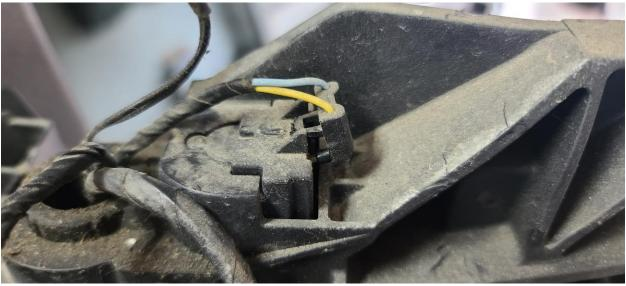
Slide the wiring through the plastic frame being careful not to bend up the motor connector pins
