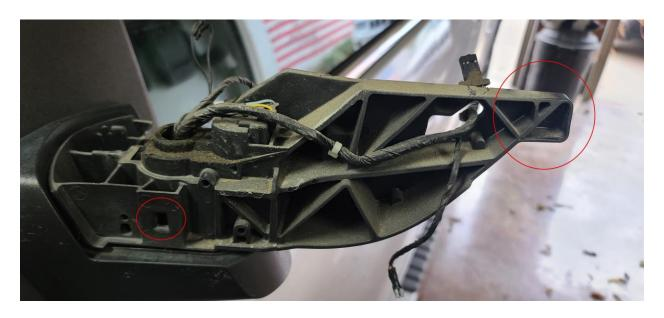
Remove frame pins with punch and hammer
