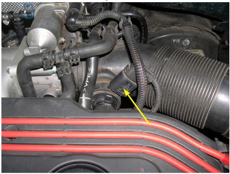
4. Disconnect the intake hose from the MAF by temporarily removing tension from the spring damp indicated by the yellow arrow in the picture below and then sliding the hose off of the MAF.
