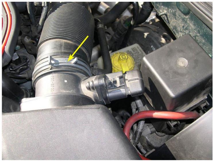
5. Move the disconnected end of the intake hose to the side of the opening in the MAF (as shown in the picture below) so that there will be unobstructed airflow during the compression test. Make sure not to drop anything into the intake hose or leave small objects or tools near the opening - you don't want anything to be unexpectedly sucked into the intake during the test!
