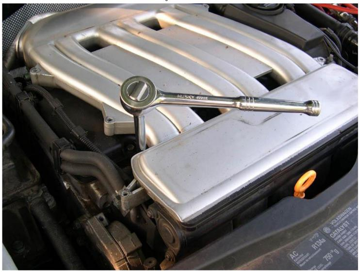
12. Disable the ignition system (make sure ignition is turned off first) by disconnecting the harness connector from the top of the coil pack on driver's side of the cylinder head. The harness connector is indicated by the yellow arrow in the picture below. If you have an early VR6 with a distributor instead of a coilpack, disable the distributor in the appropriate manner.
