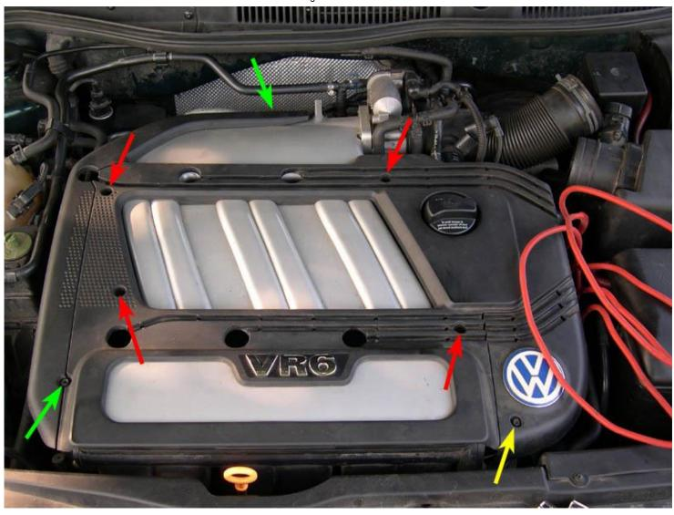
9. The plug locations and cylinder #s are indicated in the picture below (FYI, the firing order on the VR6 is 1-5-3-6-2-4).
