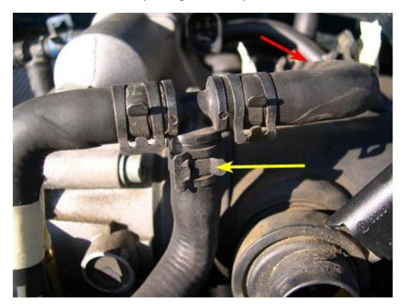
26. Release the tension from the clamp securing the main intake tube to the TB (indicated by yellow arrow in picture below) and then slide the intake tube off of the TB.
