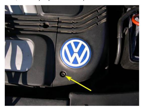
17. Remove the long, thin engine cover piece on the passenger's side of the engine by removing the two (2) T30 Torx screws indicated by the yellow arrows in the picture below.
