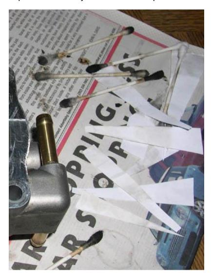
5. To clean the TB, spray the TB cleaner onto the deposits inside the TB, allow it to soak in for a few seconds and then gently scrub away the deposits with the Q-tips and/or paper towels. Using this method, you should be able to remove all of the deposits EXCEPT for those between the edge of the throttle valve and TB wall. We'll get to those deposits shortly. First, here are some VERY important warnings.
