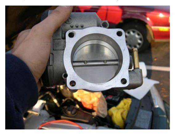
11. To reinstall the TB, follow the steps for the removal method in Part I that you used in reverse, and then proceed to Part III.
