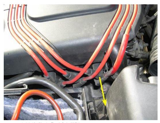
15. Unclip the spark plug wires from the channels in the engine cover, as shown below.
