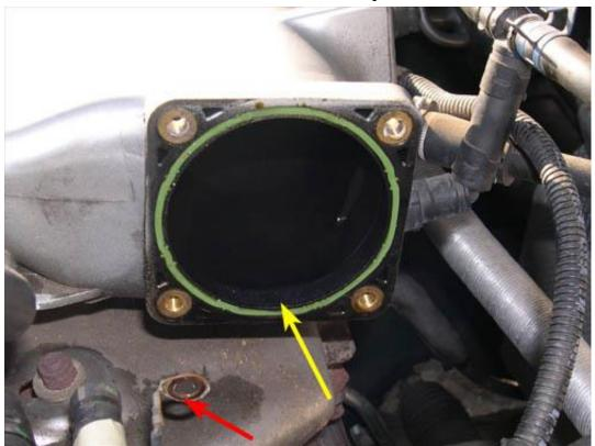
30. If you are replacing the TB, install the new unit by following steps 12 through 28 in reverse and then proceed to Part III (TB adaptation). If you are cleaning your existing TB, proceed directly to Part II.
