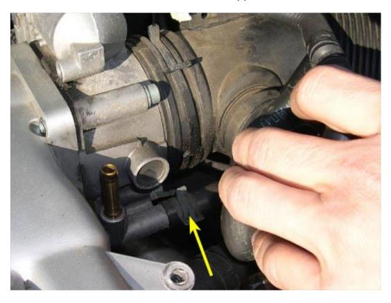
25. Disconnect the vertical coolant hose (yellow arrow in picture below) from the T-junction in front of the TB/main air intake tube. Next, unclip the horizontal portion of the coolant hose T-junction from the top of the main intake tube (red arrow in picture below) and then move the hose out of the way. At this point, there should be no coolant hoses attached to the TB, nor should there be any coolant hoses or electrical leads passing over the top of the main intake tube.
