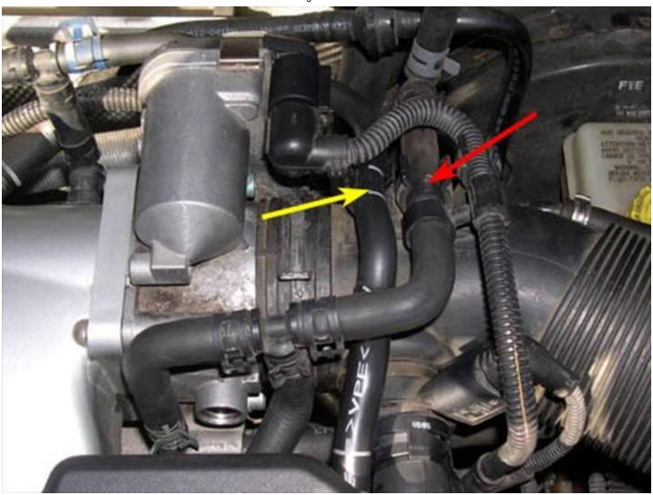
6. Disconnect the upper coolant hose (yellow arrow in picture below) and lower coolant hose (blue arrow in picture below) from the TB. To do this, use the appropriate tool (pliers or screwdriver) to release the tension from the hose clamp, slide the clamp down the hose and out of the way (for spring clamps, make sure the clamp is moved past the end of the nipple inside the hose or the clamp will reapply pressure to the nipple when released), and then pull the hose off of it's nipple.
