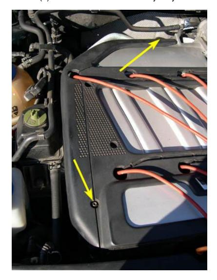
18. Remove the main engine cover piece by removing the four (4) T30 Torx screws indicated by the yellow arrows in the picture below. As you lift up on the cover piece, you will need to thread the spark plug wires through their respective holes in the cover in order to fully remove it.
