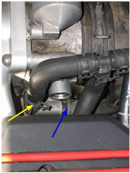
7. Release the tension from the clamp securing the main air intake tube to the TB (indicated by yellow arrow in picture below) and then slide the intake tube off of the TB.
