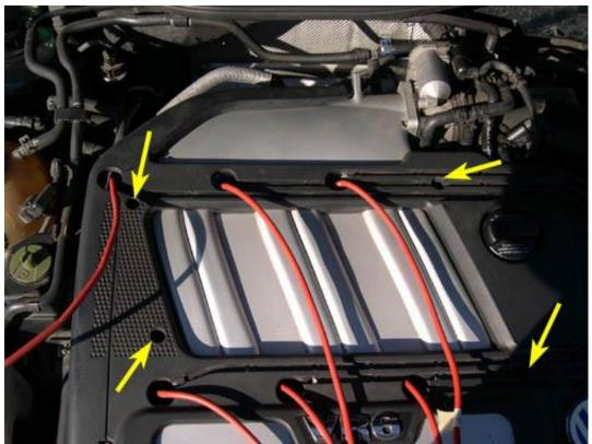
19. The picture below shows how the top of the engine should look with the three engine cover pieces removed.
