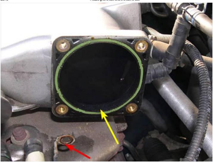
11. If you are replacing the TB, install the new unit by following steps 3 through 9 in reverse and then proceed to Part III (TB adaptation). If you are cleaning your existing TB, proceed to Part II.
