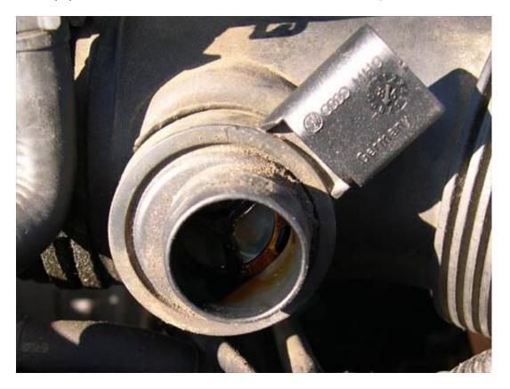
23. Disconnect the upper coolant hose (yellow arrow in picture below) from the TB. The nipple on the TB is approximately 1" long, so the clamp has to be moved up the hose at least that much in
