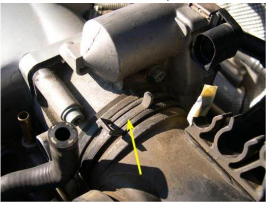
27. The picture below shows the large amount of condensed oil vapor in the main intake tube due to the PCV circuit. I wiped this oil off the inside of the tube with a paper towel. (I can only imagine how much oil is in the intake manifold and elsewhere in the engine. Someday I'll clean it all out.)
