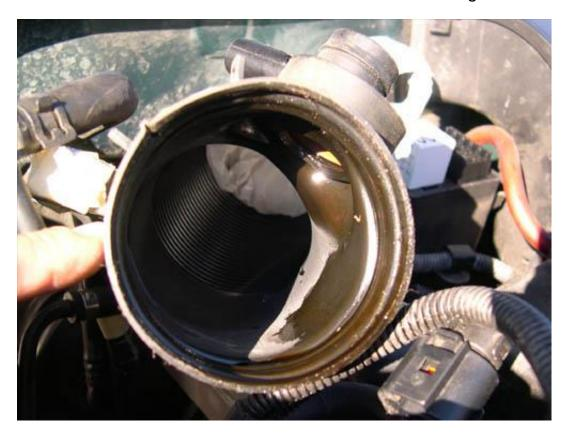
28. Using a 5mm hex/Allen wrench, remove the 4 long bolts that secure the TB to the intake
