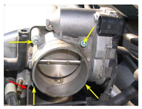
CAUTION: Be careful not to let ANYTHING fall into the intake manifold while the TB is removed. You don't want any foreign objects being sucked into the engine when it's first started - this may cause severe damage!
