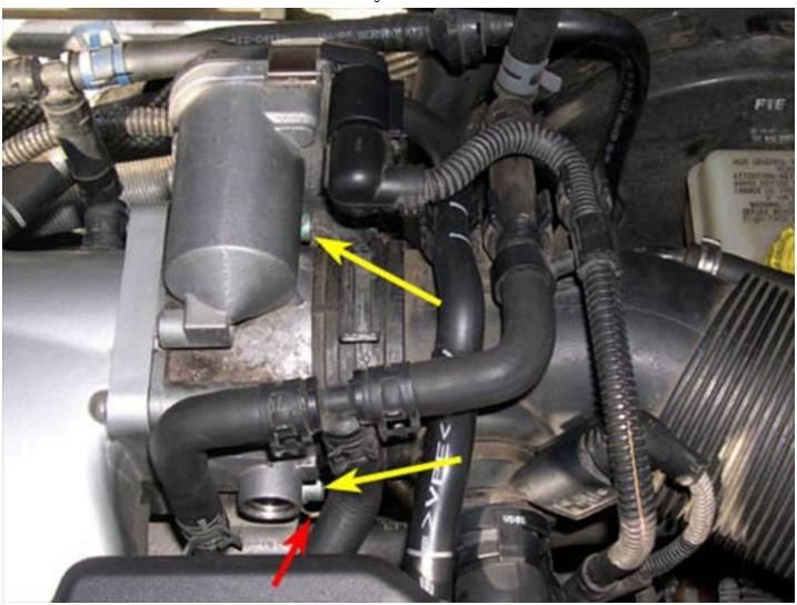
9. While holding the main intake tube and coolant/vacuum hoses out of the way, pull the TB up and off of the intake manifold.
