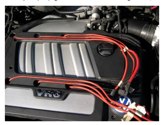
16. Remove the small engine cover piece with the VW logo on it by removing the single T30 Torx screw, indicated by the yellow arrow in the picture below.
