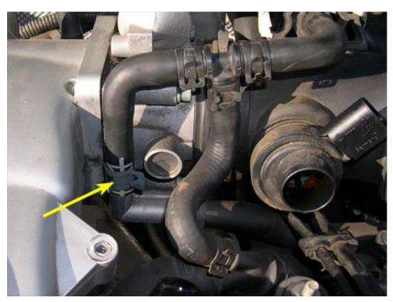
24. Disconnect the lower coolant hose (yellow arrow in picture below) from the TB. Again the nipple on the TB is approximately 1" long, so the clamp has to be moved down the hose at least that much in order to remove the hose from the nipple.
