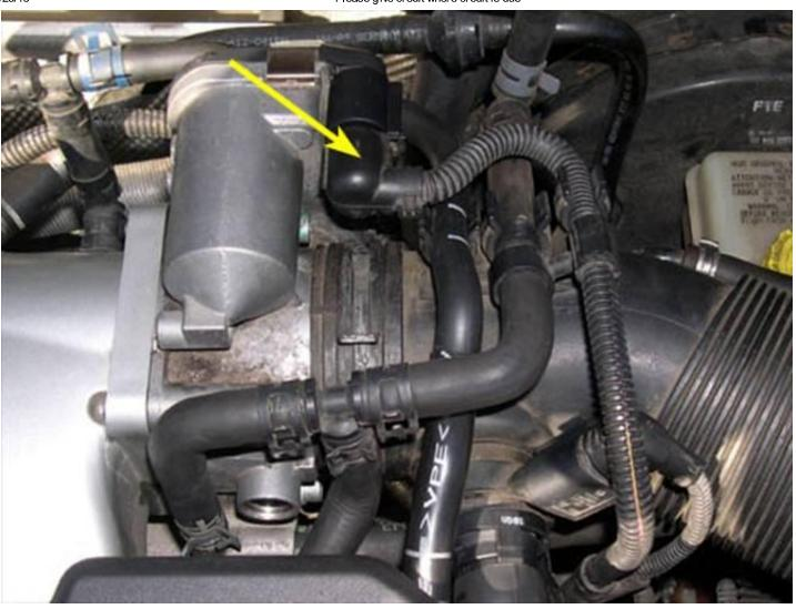
5. Unclip the coolant hose (red arrow in picture below) and the PCV vacuum-assist hose (yellow arrow in picture below) from the top of the air intake tube.
