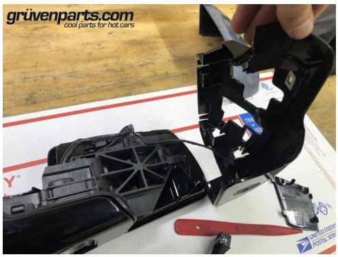
7. Unplug the electrical connector for the puddle light (if so equipped).
