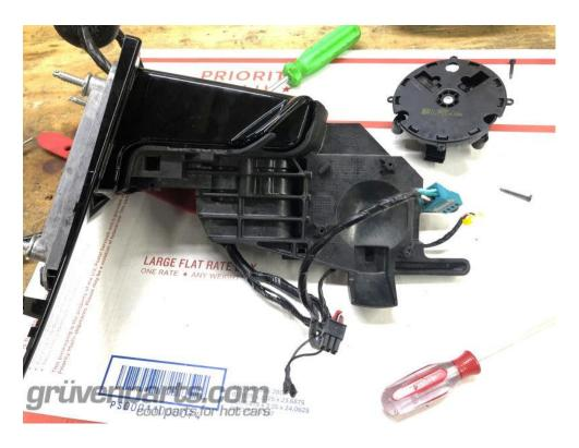
10. Working from the bottom of the mirror assembly where we removed the access cover in step 3, remove the T-15 torx screw.
