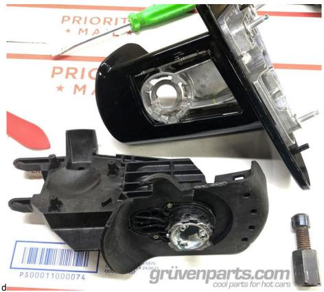
12. Remove the three T-15 torx screws which hold the power fold drive unit into the mirror assembly.
