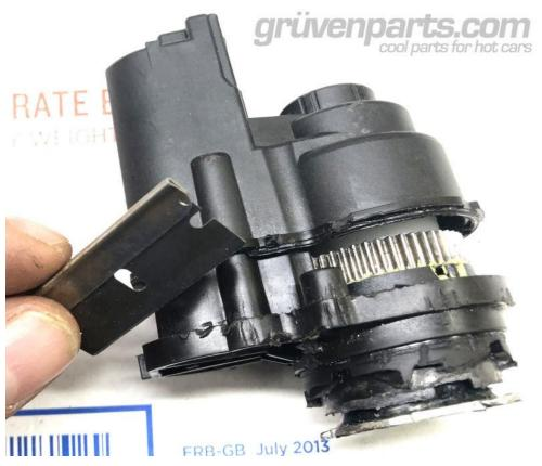
15. Separate the case halves. Now the motor, the motor circuit board, and the drive gear can all be removed. Note when you install the GruvenParts.com motor and gear, you will reuse the small circuit board so note its orientation (it will only fit 1 way). There is also a small rubber washer on the top of the motor, make sure to install that over to the new motor. There are small metal bushings that go on either side of the gear, make sure to put those on the new GruvenParts.com metal gear.
