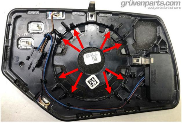
9. Unplug the mirror glass adjuster electrical connector and remove the three T-15 Torx screws which hold the mirror glass adjuster unit to the mirror frame.
