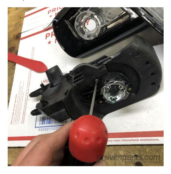
13. Remove the power fold drive unit from the mirror assembly. You may need to use a thin flat head screw drive to pry it out.
