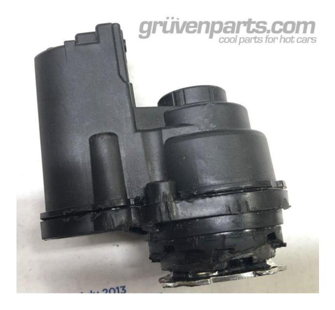
14. Use a razor or small box cutter to go around the perimeter of the power fold drive unit. They "heat seal" this unit to keep moisture out.
