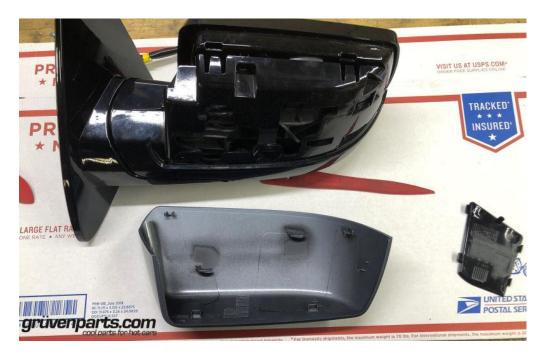
6. Now remove the underlying trim cover on the fwd side of the mirror. This has a few tabs but easily comes off. Note the 2 little fingers on the outboard end. The trim cover will rotate off as shown.
