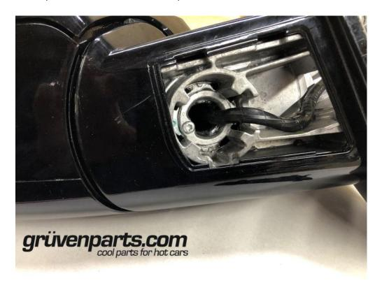
4. Remove top outer trim panel using plastic lever (trim tool). This cover will separate from the mirror housing by gently prying as shown in the picture below while pulling out on the cover.
