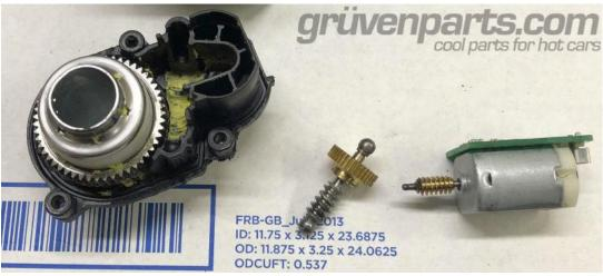
16. After installation of the replacement motor and gear, apply a thin bead of RTV sealant around the perimeter of the case halves. Reassemble the case halves and tighten down the T-15 screws. The rest of the installation is the reverse of removal.
