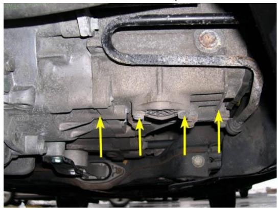
38. Jack up on the tranny very slightly, just enough to support the weight once the tranny mount bolts are loosened, not enough to actually jack up the tranny.
