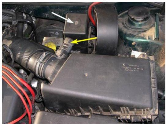
21. Unscrew the two Phillips head screws that hold the cover of the air filter box to the main section of the box. The screws are indicated by the yellow arrows in the picture below. You do not need to remove the screws completely, only unscrew them until they come out of the lower box (they can slide up 1/4"-1/2" easily when this point is reached).
