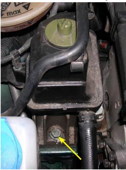
31. Remove the rear 16mm passenger's side engine mount-to-body bolt indicated by the yellow arrow in the picture below.
