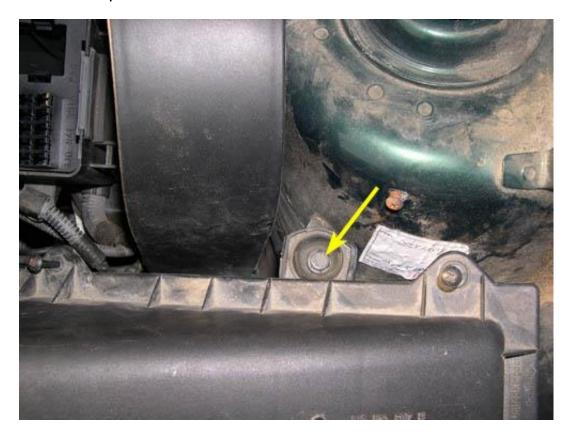
26. Remove the front 10mm bolt that attaches the air box to the car. The bolt is down between the air box and battery box - you'll need a long extension to get to it.
