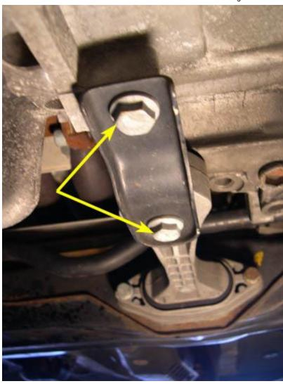
30. Remove the front 16mm passenger's side engine mount-to-body bolt indicated by the yellow arrow in the picture below.
