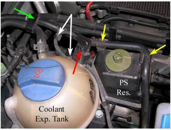
6. Disconnect the CET from the body by removing the two Phillips head screws indicated by the yellow arrows in the picture below.
