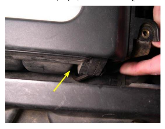
15. Move the metal coolant pipe (yellow arrow in picture below) towards the front of the car and down along side the hard, flexible hose (red arrow in picture below - part of the secondary air injection system?). This will prevent the hose, which will raise up with the engine, from pushing the coolant pipe against the A/C service valve discussed in step 9.
