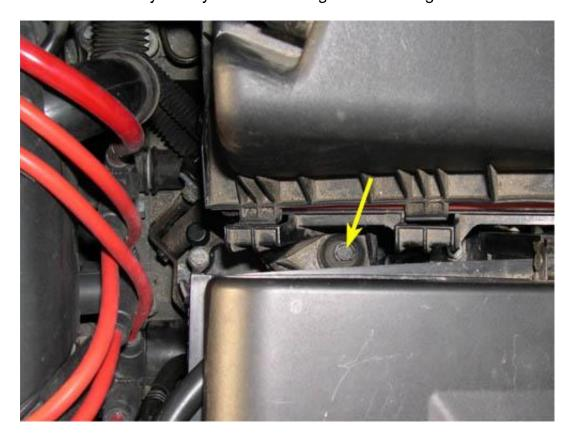
27. While holding the air box cover up and out of the way (a second pair of hands is helpful), slide the air box toward the passenger's side of the car and up and out of the car. The air box is secured on the driver's side by the intake snorkel (hole for snorkel can be seen in the picture below) and a rubber rod (yellow arrow in picture below). These make the air box difficult to remove.
