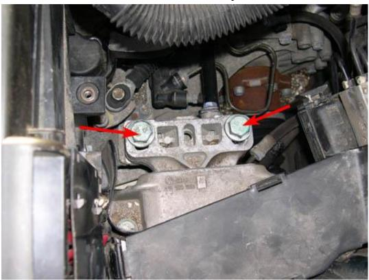
40. Push the engine/tranny over towards the driver's side as far as it will go. It may be helpful to have someone lift and pull the tranny over from the driver's side of the car while someone else pushes the engine over from the passenger's side.
