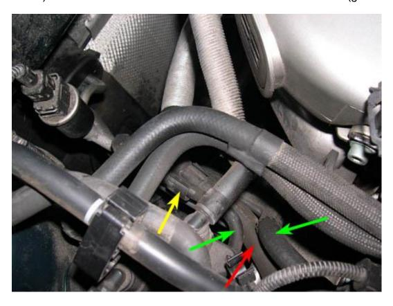
8. Remove the 13mm bolt that connects the PSR support to the body, as indicated by the yellow
