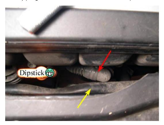
16. Remove the lower sound absorber panel from underneath the engine/tranny (red arrow in picture below) by removing the four T25 Torx screws that attach it to the car. There are two screws on each side of the panel. The two on the passenger's side of the panel are indicated by the yellow arrows in the picture below.
