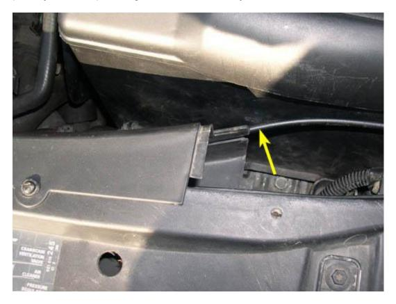
13. Remove the trim piece by removing the two Phillips head screws indicated by the yellow arrows in the picture below and sliding the piece toward the rear of the car and up and out.
