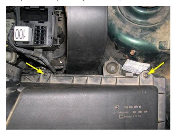
22. The other side of the air filter box cover is held down by four tabs, indicated by the yellow arrows in the picture below. To remove the cover, you need to lift up on the rear slightly (red arrow in picture below) to release the tabs and then slide the cover towards the rear of the car (green arrow in picture below).
