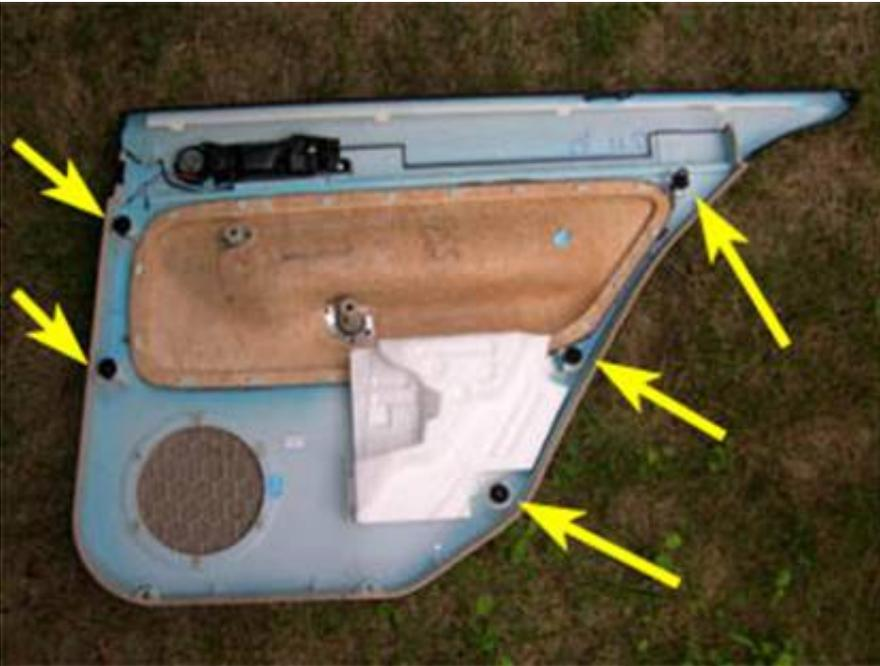
9. Starting with the top, rear corner, pull the door panel up and out of the window seal, as shown below.
