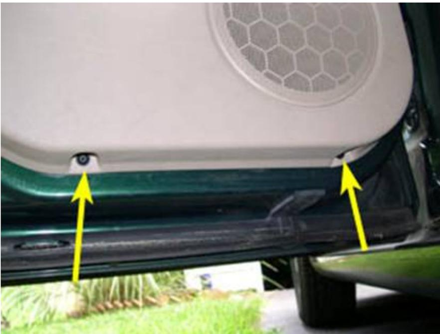
7. Starting at the bottom of the door, pull the door panel away from the door, as shown below. There are five snaps securing the panel to the door, two near the front edge of the panel and three near the rear edge of the panel. The approximate location of the two lowermost snaps on the rear edge are indicated by the red spots. After unsnapping the five snaps, the door panel should still be attached to the top of the door near the bottom of the window.
