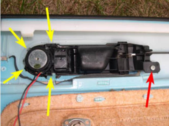
16. Once the front edge of the handle assembly is pushed out (1), slide the assembly toward the front of the car to remove (2).
