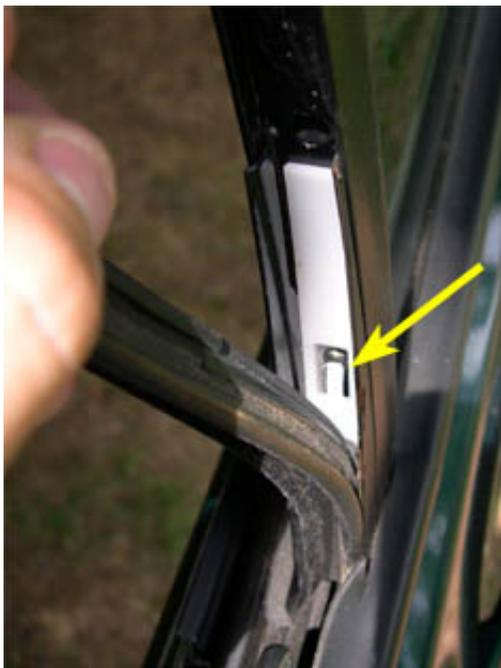
21. Using a screwdriver, pull the tab outward and simultaneously slide the insert up and out of the door, as shown below.
