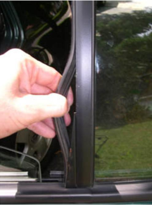
19. Pull out the seal from nearly top to bottom, as shown below, but don't remove the seal completely. Leave it attached at the top of the window and also to the bottom of the triangular insert. This will help insure that it goes back in correctly.
