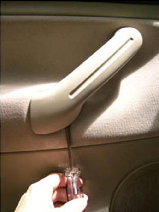
3. Once one end of the outer handle piece is pried off slightly, move to the other end and pry that out slightly, as shown below. Go back and forth between ends until the handle has been pried out approx. 1/8". Once it is this far out, you should be able to pull it off the rest of the way with your hands.
