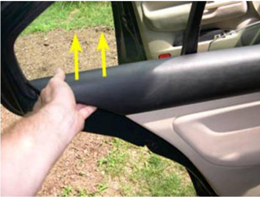
10. Do the same with the top, front corner of the door panel, as shown below. The door panel should now be disconnected from the door except for the electrical and door lock cable connections in between the panel and the door. You can rest the door panel back into the window seal if you want to take a break or reach for a tool.
