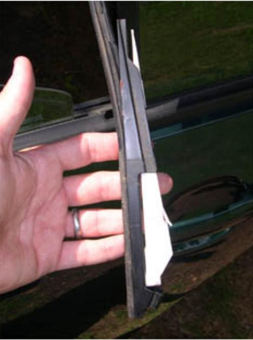
23. Take note of the position of the bottom of the rubber seal (yellow arrow) relative to that of the bottom of the insert (red arrow), as shown below. Make sure to attach the seal to the new insert in the same position so that the seal reinstalls into the quarter panel window divider correctly.
