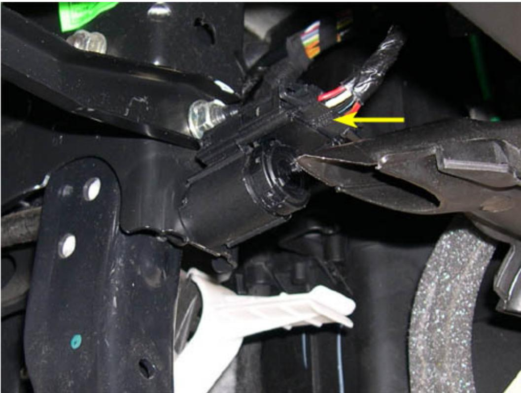
**WARNING:** If at any time during steps 5 and 6 the switch backs away from the bracket (even a little bit), DO NOT ATTEMPT TO ROTATE THE SWITCH INTO POSITION!!! It will
