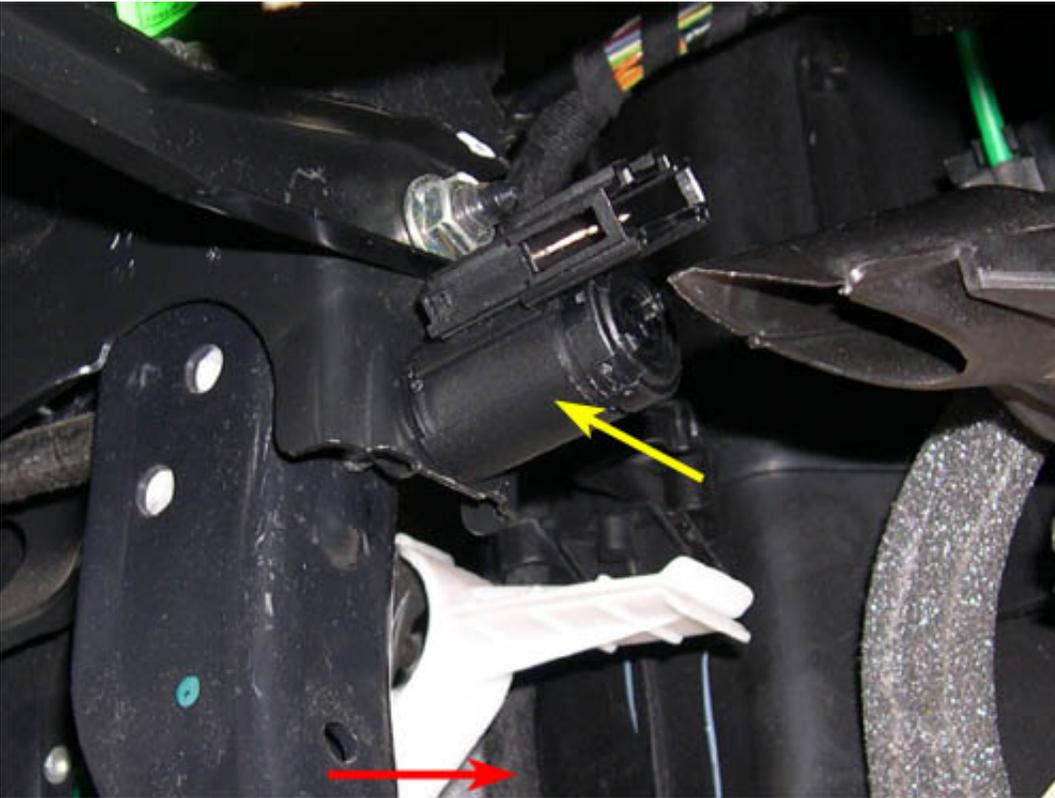
5. While holding the switch in place (DO NOT LET IT PUSH BACKWARDS - THIS IS CRITICAL), release the brake pedal and pull it back slowly as far as it will go (until it hits the stop), as indicated by the red arrow in the picture above. You should hear the plunger click as it compresses. This procedure sets the correct length for the switch plunger.
