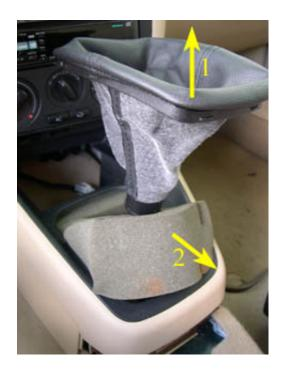
28. At this point, attempt to slide the lower center console backward, disconnecting it from the main (vertical) center console. If you are able to remove the lower center console without any difficulty, goto step 34 (ignore steps 29 through 33 - they are not applicable to your model year).
