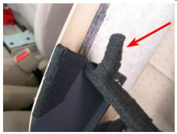
35. These fingers insert into corresponding holes in the bottom of the main center console (yellow arrows), as shown below. The fingers (above) are normally bare plastic, but I covered them with felt to prevent the fingers from rubbing in the holes - this caused a loud creaking when side pressure from my knee was applied to the lower center console while driving. This cured the problem. I recommend that you do this if you have the lower center console removed.
