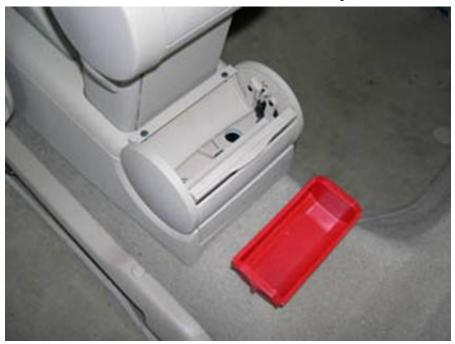
3. Remove the two sides to the rear ashtray as shown in the picture below. Pry the top of the ashtray side off of the ashtray housing (1). Once this is done, pull upwards on the ashtray side (may have to pull hard) to remove it (2).
