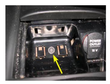
21. Using two screwdrivers (only one is shown), pull the two tabs indicated by the arrows in the picture below up simultaneously (1) and slide the ashtray toward the front of the car (into the center console) approximately 1/2" (2). Be careful to only pry the tabs up slightly as they break very easily - I managed to break the left one in the picture. They only need to come up enough to clear the metal bracket underneath that the ashtray attaches to.
