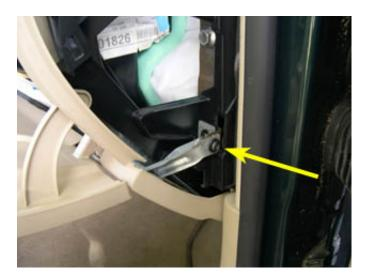
39. Use a screwdriver to carefully pry out the rear of the light in the glove box(1) and then slide it towards the rear of the car to get it out (2), as shown below.
