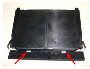
61. If you have the newer-style cupholder (the one with the spring-loaded arms, remove the flap by using a screwdriver to pop off the metal tabs that secure it to the main cupholder unit, as shown below.
