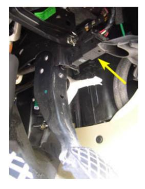
50. To disconnect the brake light switch from it's harness connector, push the two tabs (indicated by arrows in the picture below) toward each other and pull the harness connector off of the switch.
