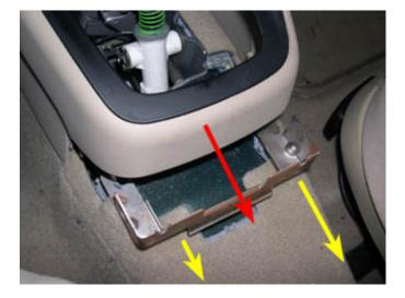
34. The lower center console has two plastic fingers approx. 1.5" long which protrude from the front edge (red arrows in picture below points to driver's side finger).
