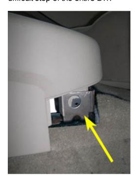
30. Begin by removing the 10mm nut (right) which holds the bracket down, as shown below.
