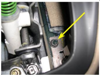
31. The lower center console sits directly above the nut, so a flex-joint socket or something similar is needed to remove the nut. I put a 10mm socket onto the nut and then used a socket driver which was not fully inserted into the socket and at an angle to remove the nut (see picture below).
