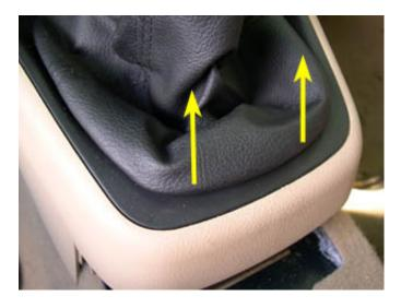
27. Slide the boot all the way up and out of the way and remove the foam piece that surrounds the
