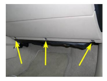
42. Remove the three T20 Torx screws on the top of the glove box, as shown below. Pull the glove box out and disconnect the microswitch for the glove box light from near the driver's side hinge. The glove box can now be removed from the car.
