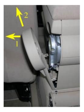
9. Be careful doing the above. The trim piece is held in by 6 tabs as shown in the picture below (arrows). I've removed this piece enough times that I've partially broken one of the tabs (red arrow). You can use a thin screwdriver protected by a thin rag to help ease the tabs out.
