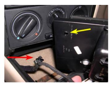
24. Disconnect the power wire from the 12v outlet by pressing in the white tab (1) and pulling the
