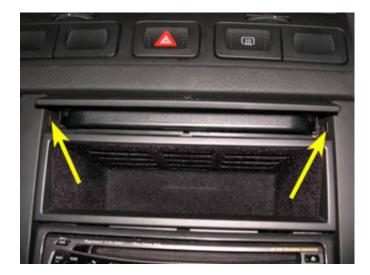
58. The picture below shows one of the clips that secures the cupholder in place.
