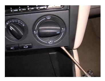
56. Remove the four T20 Torx screws at the corners of the HVAC controls, as indicated by the arrows in the picture below.
