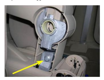
11. Remove the two T20 Torx screws indicated by the arrows in the picture below.
