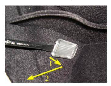
40. Disconnect the harness connector from the light by pulling the two tabs apart simultaneously, as shown below. Once disconnected, push the wire back into the hole that the light occupies.
