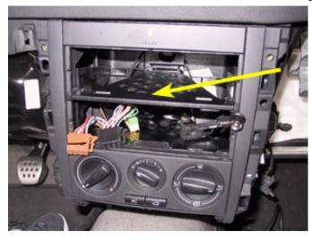
54. The DIN support tray is secured with a clip on either side (yellow arrows in picture below) and a tab at the rear (red arrow in picture below). Undo the clip on both sides of the tray (may need to use a screwdriver or other tool - I can't remember) and then pull the tray out to disconnect the tab at the rear.
