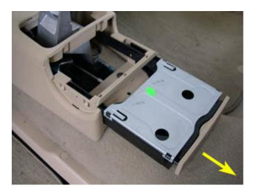
8. Remove the driver's side of the armrest trim as shown in the picture below. First pull the top of the trim towards the driver's side (1) and then pull upwards at an angle to remove (2).
