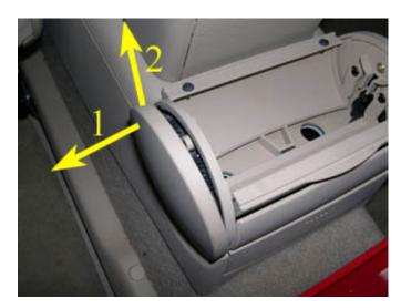
4. The picture below illustrates how the top and bottom of the ashtray sides are connected to the ashtray.
