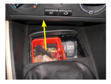
19. Remove the small trim piece just below the A/C controls (or Climatronic if that's what you have) by pulling it towards the rear of the car, as shown below. While this step is not absolutely
